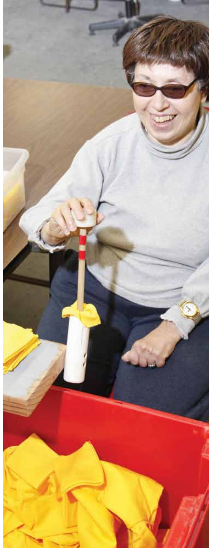
After the jig was in place, the cuff was placed on it and inverted by placing a rod through the jig.
