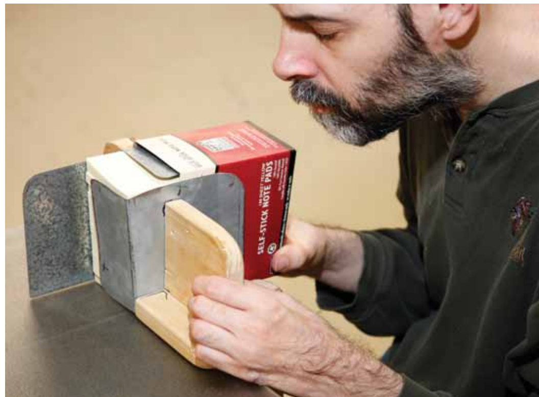
At ABVI-Goodwill Industries, Rochester, New York, NIB rehabilitation engineers designed and built a jig for packaging 3M memo pads to enable David Sayre to perform the standard packaging procedures.
