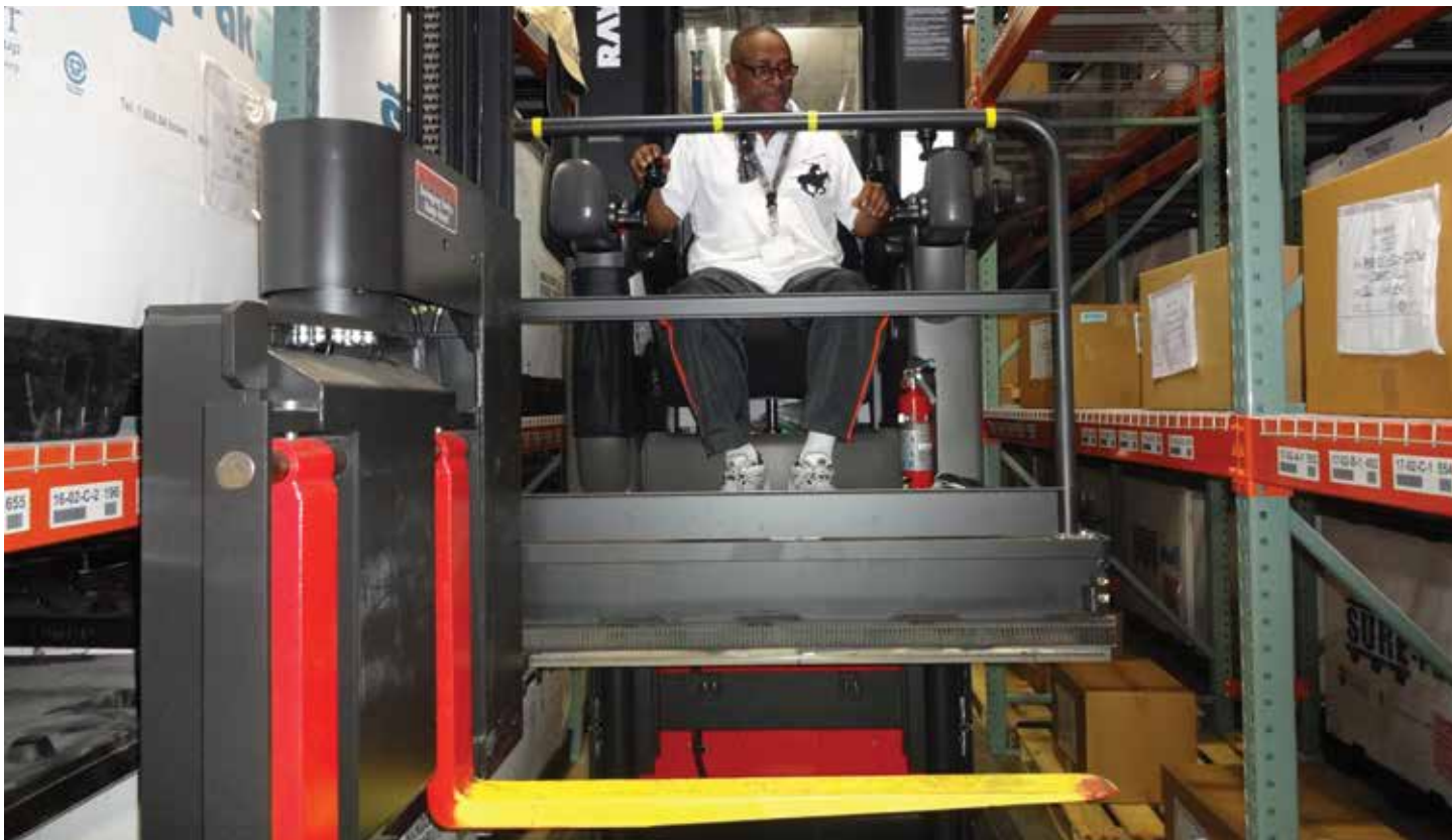
▲ Bright yellow paint provides maximum color contrast on a turret truck operated by Schubert Whitaker, warehouse specialist and forklift operator, Travis Association for the Blind, Austin, Texas.
